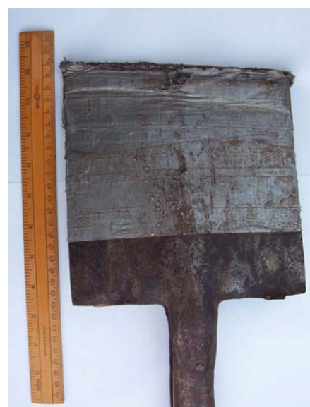
Lifting Spade with Protective Tape
