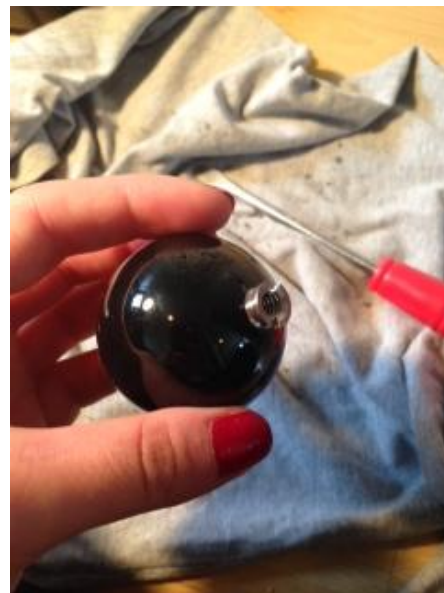
Fig.2 Fixing a 1/4" threaded nut to the ball
