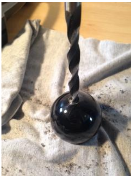
Fig.1 Drilling a snooker ball with a 1/4" drill.
